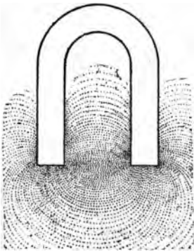
FIG. 24.—Lines of force of a "horseshoe" magnet.
